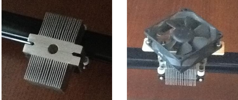
Heat sink made from a spare aluminum CPU heat sink
